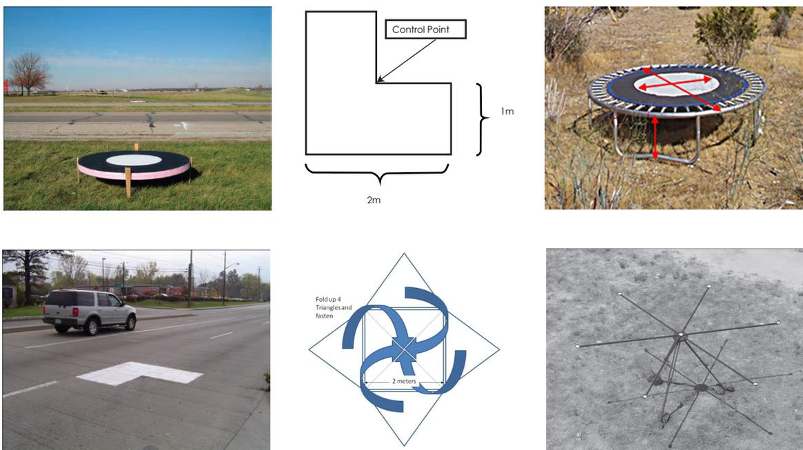
Figure 1 Targets used in planimetric and vertical elevation assessment of lidar data.
