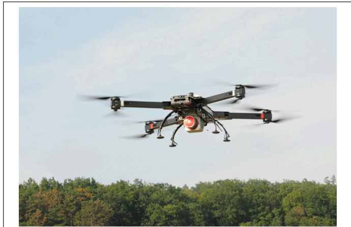
Figure 9. Riegl's entry into the unmanned aerial vehicle market is an extension of its long-term multisensory approach. The company's first foray into midrange TLS—the LMS-Z160/Z210—was made possible by its work with the ESA for shuttle landing sensors. Distance-sensing technology from its preexisting portfolio of instruments was also modified to create its new laser scanning sensor.
