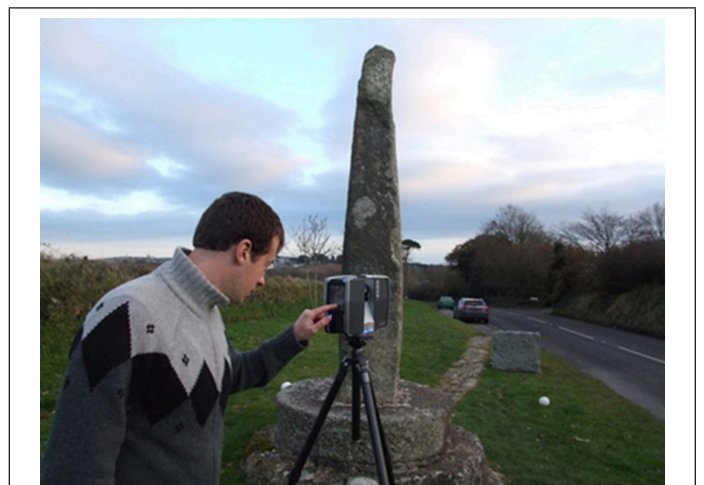
Figure 3. Checkerboard targets, crosshair black-and-white targets, and matte white spheres are used as targets in midrange TLS when the laser beam is set to a certain wavelength. The first-generation FARO Focus 3D —here being used to document the Tristan Stone, a medieval inscribed stone in Cornwall, UK—is set to a 1550-nm wavelength on the electromagnetic spectrum. Not all laser scanners are set to the same wavelength. The dynamic range of the information returned to the scanner can also be taken into account, as discussed in the section “Laser Scanning in Its Commercial Era (from 1979 Onward).”
