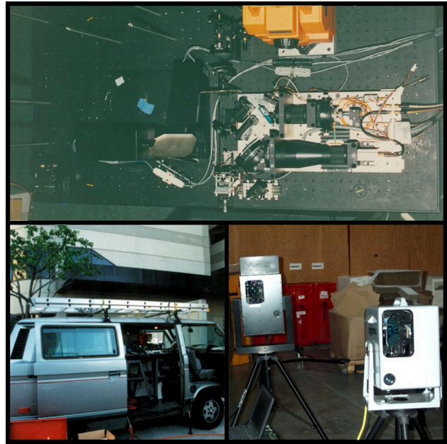
Figure 8. Early stages of development for the Cyra scanners from Cyra Technologies. All photographs were kindly provided to the author by Dr. Jerry Dimsdale (Top: Email to author, January 10 th , 2020; Bottom: Email to author, March 27 th , 2013). The top photograph is of the early bench prototype for what was initially described as the Field Digital Vision machine (Wilson et al. 1999). It did not include the time-interval interpolation circuit from Los Alamos National Laboratory at this point, although the green laser from Massachusetts Institute of Technology’s (MIT) Lincoln Laboratory was in use. (Prior partnering with the MIT Lincoln Laboratory, Dimsdale and Ben Kacyra visited numerous experts in the field of laser scanning, including at the Environmental Research Institute of Michigan and the CMU Robotics Institute.) Instead, a larger box pulse generator from Stanford Research Systems was used. The unit was fitted into a Volkswagen Vanagon to make it portable (bottom left). Once the time-interval interpolation circuit had been repurposed to reach the required rate of picoseconds, the hybridized system architecture of the 532-nm green laser from the MIT Lincoln Laboratory and the Los Alamos National Laboratory time circuit were used in the smaller Cyra HDS 2400 and HDS 2500 systems (bottom right). This was prior to the 2000 acquisition of Cyra Technologies by Leica Geosystems, toward the end of the dot-com boom.
