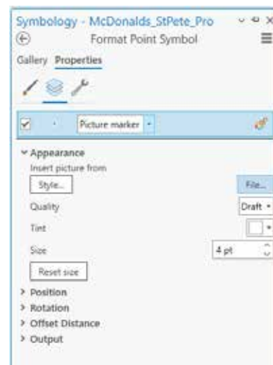
Figure 3. The Picture marker dialog box allows you to select a picture marker and manipulate the properties in ArcGIS Pro.
