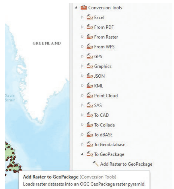
Figure 9. Adding a raster to the GeoPackage from the Conversion Tools | To GeoPackage toolset.
