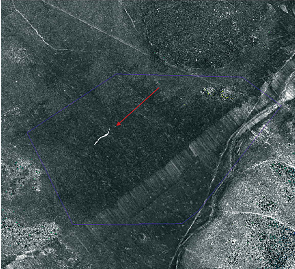
Figure 7. Poor Ground Classification Identified by High SDASN Values.
