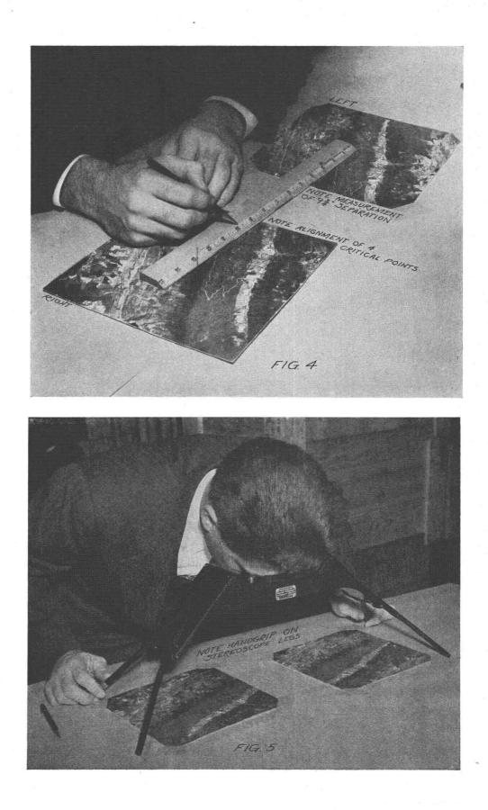
of Scotch tape or thumb tacks, fasten the left-hand photograph permanently in this position. Then rotate the right-hand photograph underneath the straight-edge in a similar fashion until the transferred principal point of that photograph is directly under the edge of the straight-edge. Then fasten the right-hand photograph securely to the drawing board and the orientation of the photograph has been accomplished. The needles can now be withdrawn.
