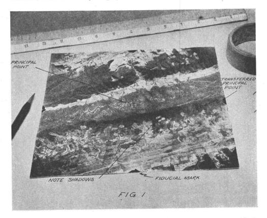
will cast shadows and these shadows will be visible to a certain extent. If high hills or mountains are in the photographs, the shadows will be apparent on the slopes of the hills away from the sun. Lay one photograph of the pair on the table so that the shadows appear to be cast by a light somewhere out beyond the upper left-hand corner of the photograph. This orientation is shown in Figure 1.
