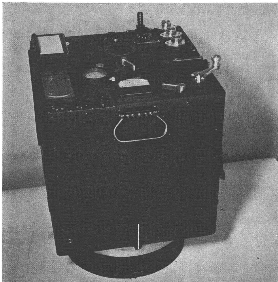
FIG. 7. AAF Type T-5 topographic camera; manual or electrical operation, 24-V; 6" f/6.3; shutter speeds 1/50th, 1/100th, 1/200th, 1/300th, between-the-lens shutter; negative size 9½"×150"; No. of exposures 190; weight of camera loaded, no filters or cables, 84.5 pounds. This camera has a built-in viewfinder, intervalometer and exposure meter; automatic recording of altitude, time, and data card made during each exposure.
