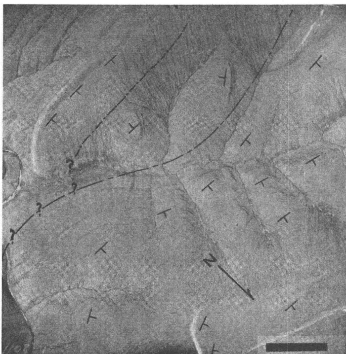
FIG. 2. Six inch focal-length vertical photograph taken at 12,000 feet with the central camera of a trimetrogon unit. During stereoscopic examination, symbols are placed on each photograph prior to transfer to the base map. Dashed lines show the axis of a sharp anticline and a small syncline depicted on the photogeologic map at Latitude 68^{\circ} 45' North, Longitude 152^{\circ} 55' West. The white outcrops are bentonite beds. (Photo courtesy—U. S. Navy.)
