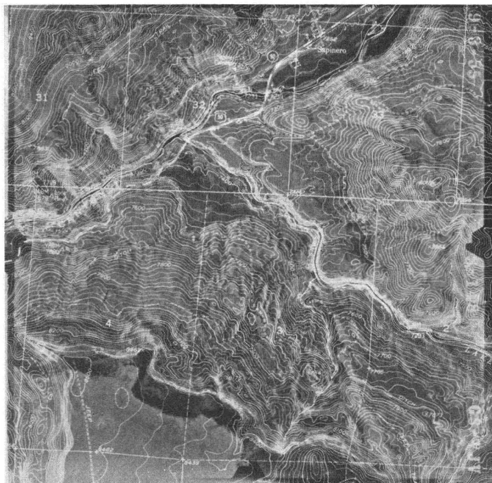
FIG. 1. Perspective aerial photograph with superimposed U.S.G.S. map. The scale of the map overprint is equal to that of the photograph at the datum of the river (upper left corner). Note the lack of scale uniformity of the photograph as exhibited by the discrepancies between the photographic features and their plotted positions on the map.
