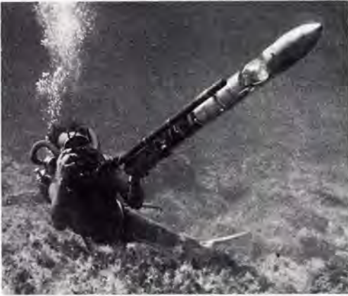
FIG. 7. Dimitri Rebikoff with his first underwater stereo "pressure cooker" camera with "torpedo strobe" oil-filled lighting system in 1950.
