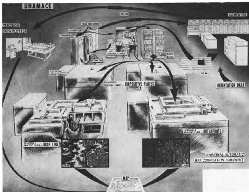
FIG. 4. The UNIMACE—Universal Automatic Map and Compilation Equipment.
