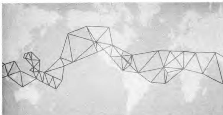
FIG. 2. SECOR (Sequential Collation of Range), a system of satellite geodesy, has nearly completed an equatorial network.
