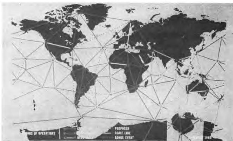
FIG. 3. TOPOCOM and the U. S. Coast & Geodetic Survey are currently in a collaborative program comprising a 46-station global network using 15 sets of BC-4 camera equipment.
