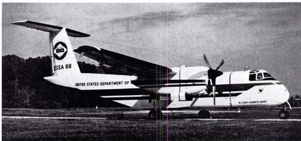
FIG. 1. NOAA-NOS Buffalo aircraft is normally equipped with three aerial cameras for simultaneous operation, or two aerial cameras and one thermal infrared mapper.
