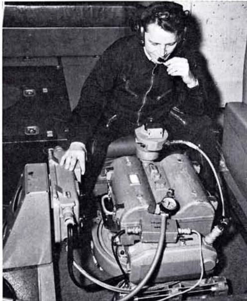
FIG. 2. Wild RC-8 camera installation on Buffalo aircraft being checked prior to commencement of photography.
