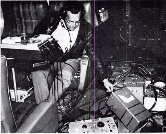
FIG. 3. Thermal infrared scanning equipment installed in Buffalo aircraft.
