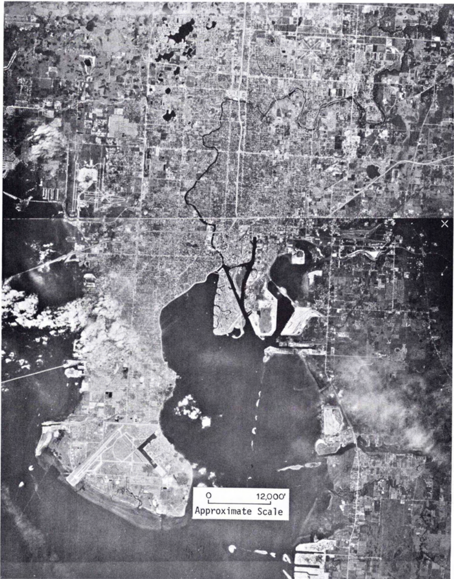
FIG. 1. A black-and-white reproduction of a 1:120,000-scale color-infrared photograph. Two photographs were spliced together in order to center on the city of Tampa, Florida. Through interpretation of this photograph the city was divided into 10 waste source areas. Number of buildings within each waste source area and the areal size of each area was then computed. Using available waste multipliers, estimates of solid waste quantities for each waste source area were made. Waste multipliers assigned an average quantity of waste per unit of time to each waste source unit, e.g., tons of waste generated per single-family dwelling per year.
