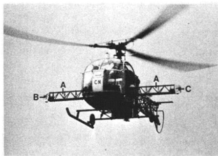
FIG. 6. Stereocamera in a helicopter taking photographs for a forest inventory. (A: Base beam, length 4.5 m; B, C: Hasselblad cameras 500 EL)
