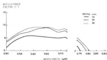
FIG. 3. Spectral response of a black plate submerged at different depths in turbid water.
