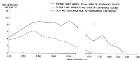
FIG. 1. Spectral characteristics of turbid river water and clear lake water.
