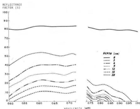
FIG. 2. Spectral response of a white plate submerged at different depths in turbid water.
