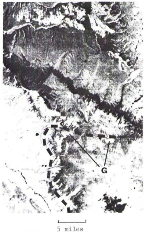
FIG. 4. Part of Landsat frame 2187-17080 (band 7), showing Cerro Summit landslide region (Montrose quadrangle). From ground truth: G—gravel terraces; broken line represents western and northern boundaries of landslide.
