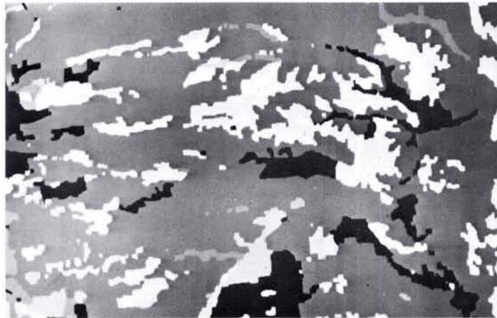
FIG. 8c. Land-use map classification processed by cleaning algorithm with parameter L = 4 .
