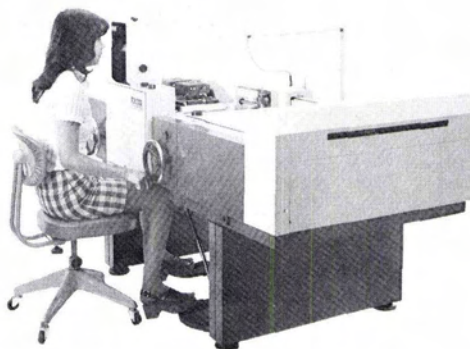
FIG. 6. Nikon TR-2 stereoplotter for police use (photo courtesy Nikon Nippon Kogaku, Tokyo, Japan).
