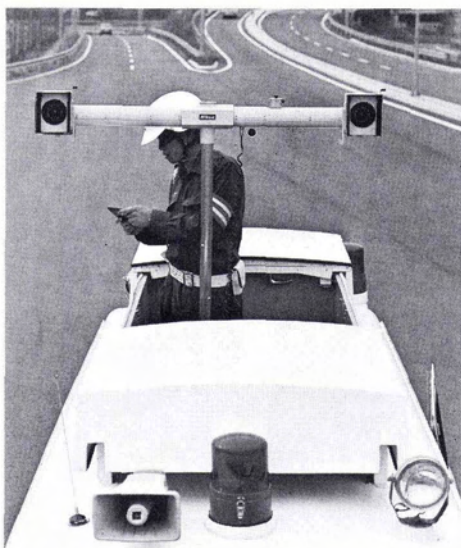
FIG. 1. Top view of a Japanese Accident Disposal Vehicle (photo courtesy National Police Headquarters, Tokyo, Japan).
