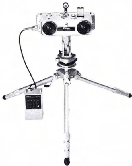
FIG. 4. Nikon TS-20 stereometric camera (20 cm base) for police use on a tripod (photo courtesy Nikon Nippon Kogaku, Tokyo, Japan).
