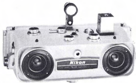
FIG. 5. Close-up view of the Nikon TS-20 stereometric camera (photo courtesy Nikon Nippon Kogaku, Tokyo, Japan).
