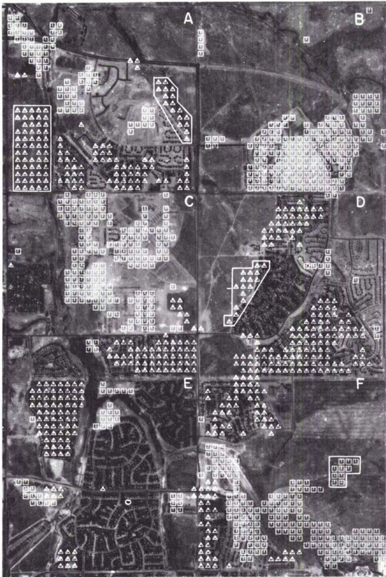
FIG. 7. A land-use change map produced using the band 5 image differencing method. The results are superimposed on the 15 October 1978 aerial photography. The two symbols represent pixels found in the lower or upper tails of the change histogram. Somer errors of commission are outlined.
