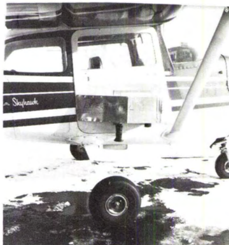
FIG. 1. Camera mount installed on a Cessna 172. Leading edge fillet (rounded, forward-most section) and trailing edge fillet (wedged, rear-most section) streamline the box shaped camera compartment (middle section).
