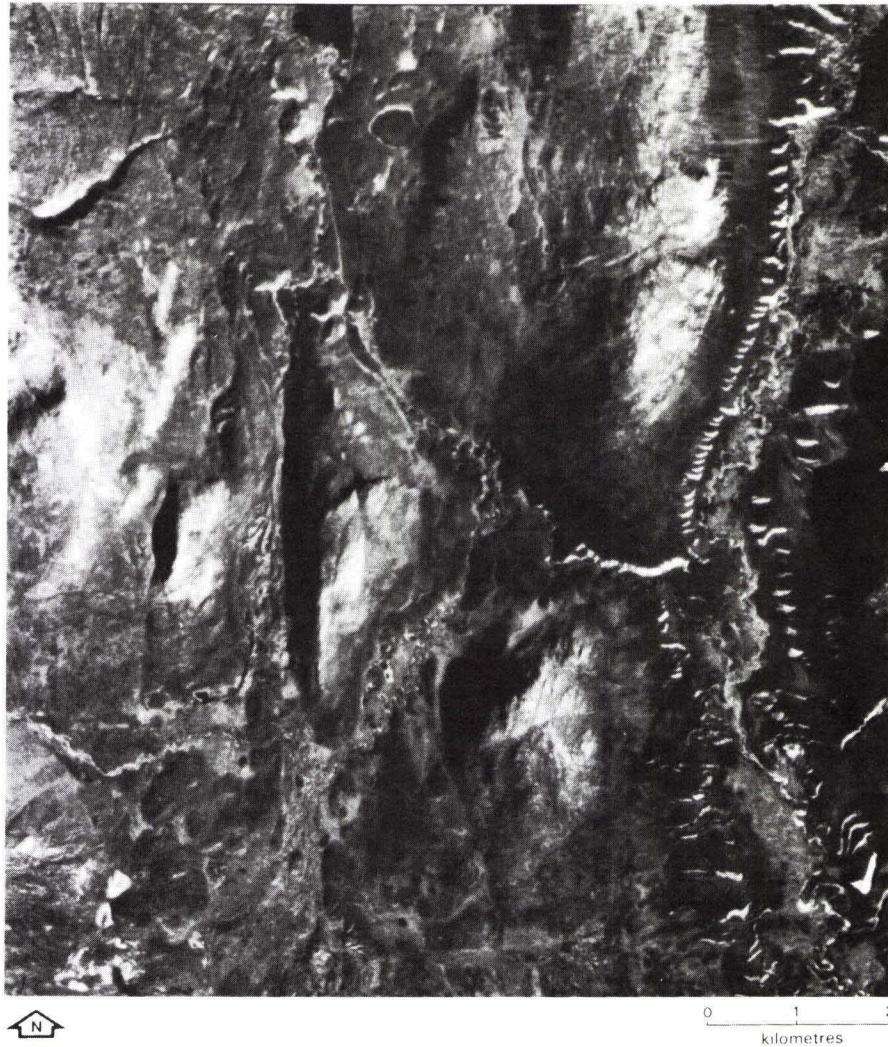
FIG. 2. Orthophotograph of the study site. The image area is approximately 9.8 km by 10.1 km. The orthophotograph was generated from metric aerial photography, acquired in August 1979, using the Gestalt Photomapper II spatial correlation machine. Locational error is less than 12 m (determined from 18 ground control points at the time of model generation). North is to the top of the image.
