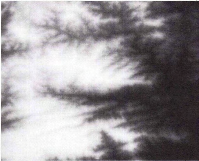
FIG. 6. 8-bit display of the USGS DEM. Elevations are represented by light (high) to dark (low) gray values.
