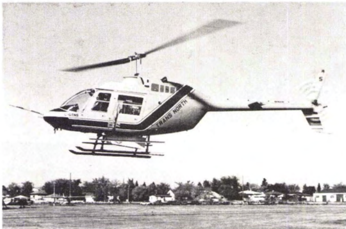
FIG. 7. Single-camera sequential system and tracking camera mounted in external camera pod, Northern Forestry Centre, Edmonton.
