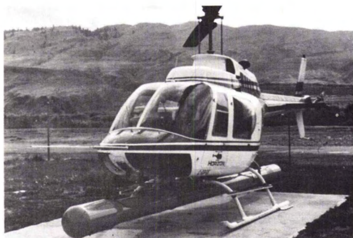
FIG. 3. Longitudinal fixed-base photo system, Timberline Ltd., Vancouver, B.C.
