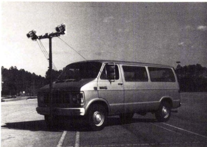
FIG. 1. The photographic collection system for pavement analysis.
