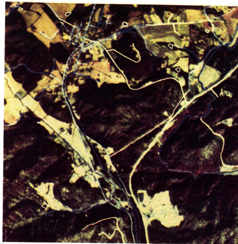
PLATE 3. Revised image map of the Tiger test area. Photo red, green, and blue image bands are shown. Original map data have been combined with the blue band while the revised data were combined with all three bands and thus appear white in the image map.
