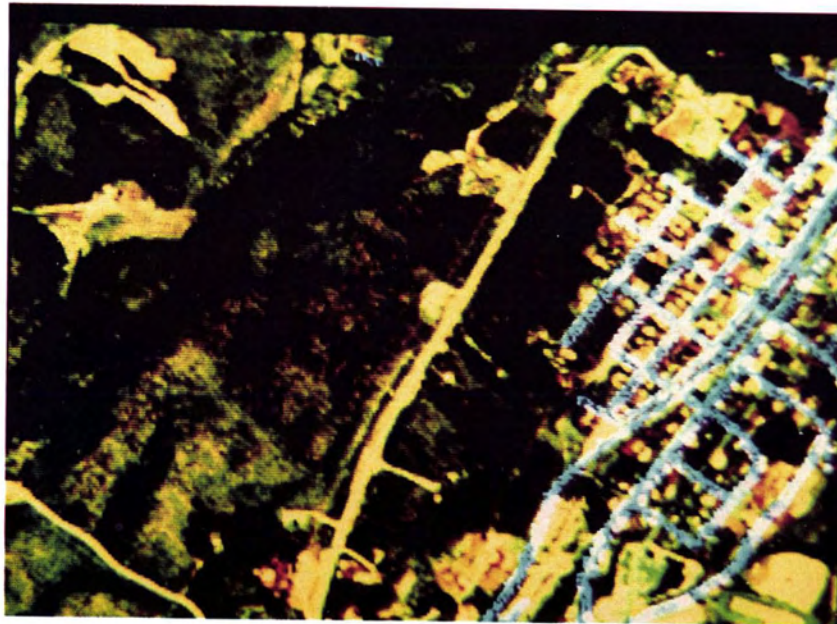
PLATE 2. Changes from the original map data to the current photographic data are easily detected by visual methods. The photographic red and green bands are shown in the red and green color memories while the map data are shown in the blue color memory.
