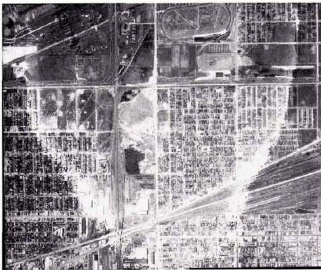
Figure 1. Contact print made from nitrate-based negative of Cicero, Illinois taken by the U.S. Army Corps of Engineers in 1933. The bright band in the center of the photo is where the negative becomes bonded with the surrounding emulsion of the roll as the nitrate-base becomes unstable.
