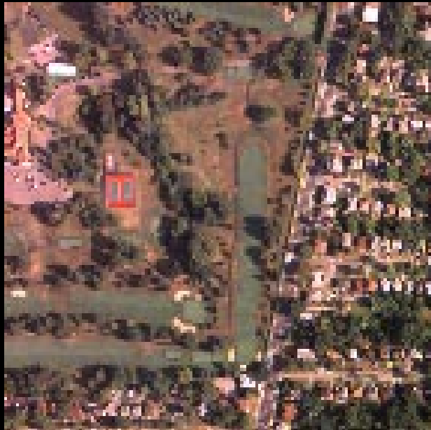
FIGURE 1. 800 pixel x 800 pixel portion of a digital orthoimage with 0.6-m (2 foot) collection and product GSD. The image was acquired with a 28 mm lens and a CCD array pixel size of 0.009 mm at an altitude of about 1800 m AGL over Cincinnati, Ohio.
