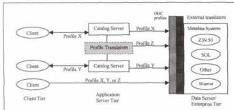
Figure 1. Approach for distributed search across distributed computing platforms.
