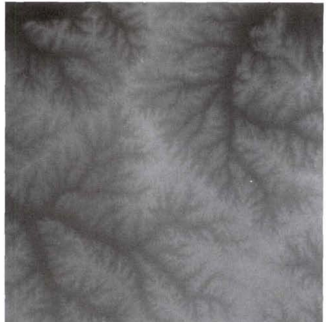
Figure 4. The gray-scale illustration of the FIFE area used in the experiment. The dark area is lower than the bright area. The minimum elevation in this area is 309 m. The maximum elevation in this area is 463 m.
