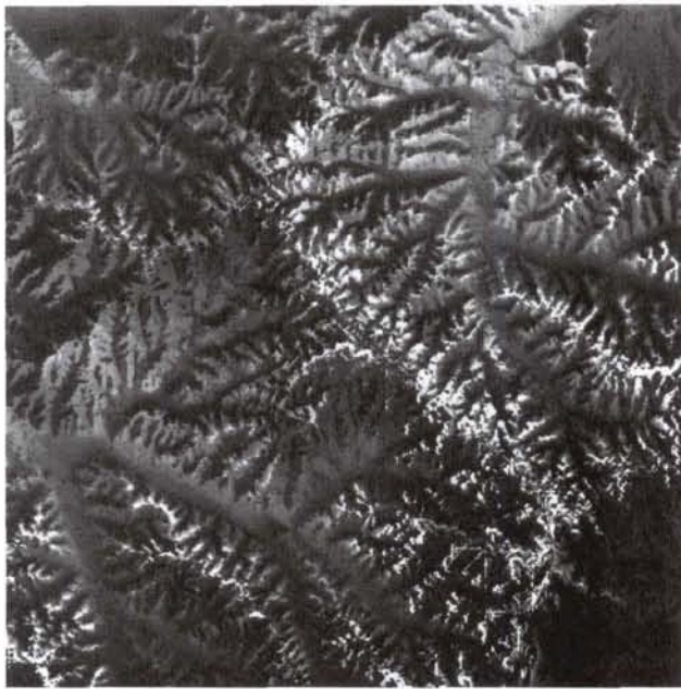
Figure 6. The gray-scale illustration of the visibility index of FIFE area. The dark area has a lower visibility than the bright area. The minimum visibility is only five grids. The maximum is 78,774 grids. The visibility is linearly scaled to the grey range from 0 to 255 in this figure.
