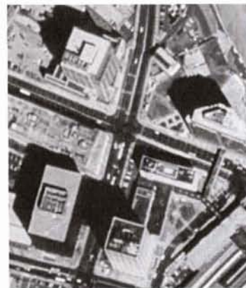
Figure 5. Oclusions due to relief displacement.
