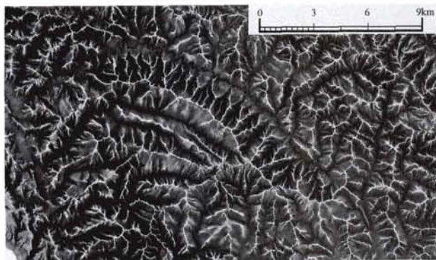
Figure 11. Positive openness ( L = 500 m) for an area south of San Francisco, California (N37:10:03 - N37:17:43, W122:06:01 - W122:22:1) computed from a 30-m DEM of the U.S. Geological Survey (USGS).
