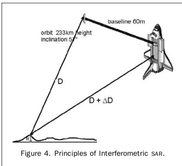
Figure 4. Principles of Interferometric SAR.
