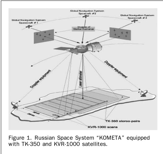
Figure 1. Russian Space System "KOMETA" equipped with TK-350 and KVR-1000 satellites.
