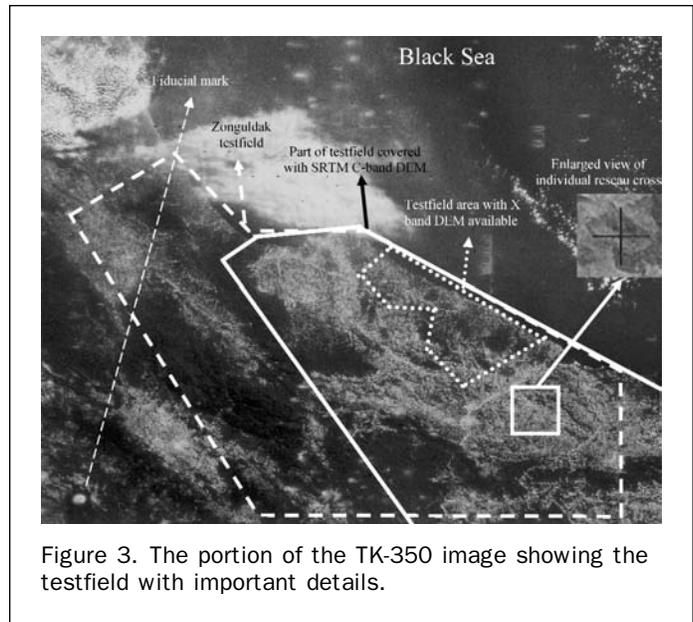
Figure 3. The portion of the TK-350 image showing the testfield with important details.
