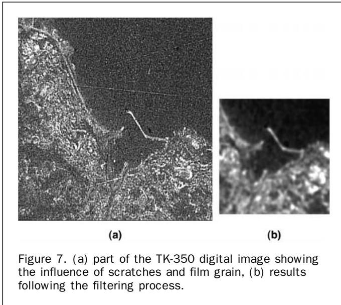
Figure 7. (a) part of the TK-350 digital image showing the influence of scratches and film grain, (b) results following the filtering process.
