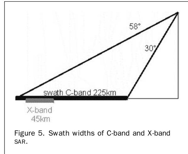
Figure 5. Swath widths of C-band and X-band SAR.
