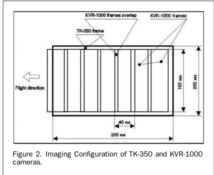
Figure 2. Imaging Configuration of TK-350 and KVR-1000 cameras.
