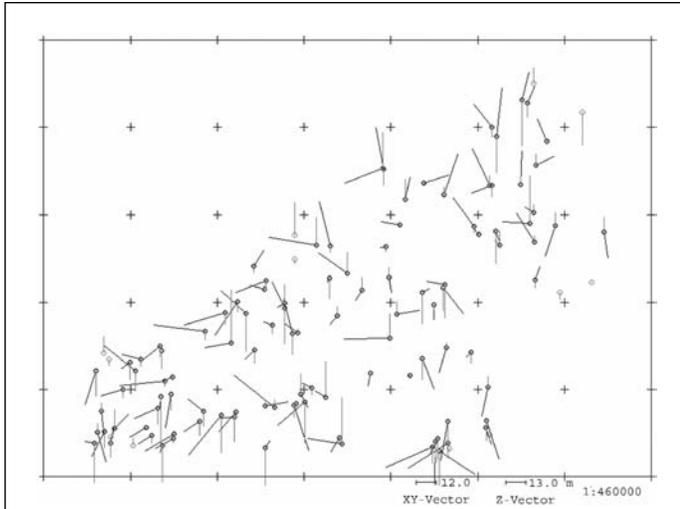
Figure 6. Vector plot of residual errors obtained from the PCI processing.
